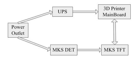
2.When system fails to connect with power, outage detection module will automatically inform touch screen that enters into printing suspending status. Power supply of UPS will depart print head from module.
